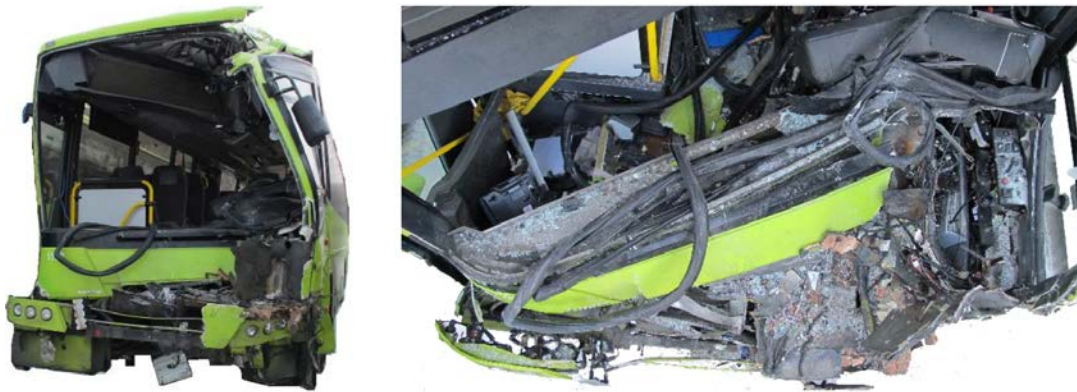
Figure 6.1: Damages to the front of the Eastgoing bus in the Nafstad accident in Norway, November 2017. Source: Accident Investigation Board Norway (AIBN) (AIBN Report Road 2019/04). Left picture from the front and right picture shows the damage to the bus front seen from above.
